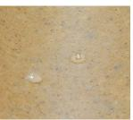
Thanks to **ACO polymer concrete**, a material with a water penetration depth of 0 mm, the entire channel run is watertight.
