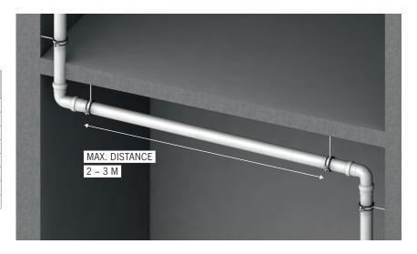
Horizontal pipework should be supported by pipe brackets in 3 meter intervals maximum. One bracket should be within 300 mm of the pipe joint and the other approximately at the midpoint of the pipe length, but not more than 3 metres from the next bracket (depending on the pipe diameter- refer to the upper table). Additional brackets should be used at changes
